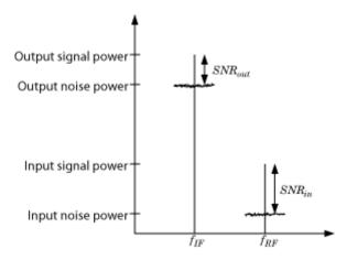
The preceding figure illustrates the effect of the receiver on the signal. The receiver amplifies a low-power RF signal at the carrier  $f_{RF}$  with a high SNR and downconverts the signal to  $f_{IF}$ . The noise figure (NF) of the system determines the difference between the SNR at the output and the SNR at the input:
