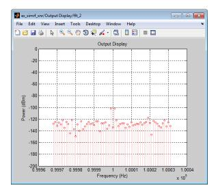
The measured PSD of -102 dBm/Hz for each tone is consistent with the 40-dB combined gain of the amplifier and mixer. The noise PSD in the figure is shown to be approximately 50 dB higher at the output, due to the gain and noise figure of the system.
