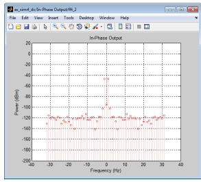
In the figure, DC power is a direct result of the blocker and the IP2 in the mixers.
