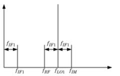
The preceding figure illustrates two input signals at the carriers  $f_{RF}$  and  $f_{IM}$  that both differ from the LO frequency,  $f_{LO1}$ , by an amount  $f_{IF1}$ . Mixing translates both input signals down to  $f_{IF1}$ . Perfect image rejection in the final stage of the receiver removes the image signal from the output entirely.
