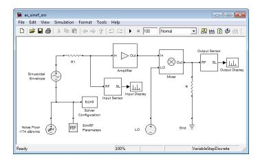
The amplifier contributes 40 dB of gain and a 15-dB noise figure, and the mixer contributes 0 dB of gain and a 20-dB noise figure, which are values characteristic of a relatively noisy, high-gain receiver. The two-tone input has a specified level of .1  $\mu$ V. A 1-V level in the local oscillator ensures consistency with the formulation of the conversion gain of the mixer.
