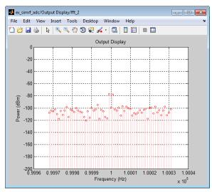
The figure shows that the receiver noise is 16 dB above the quantization noise floor.
