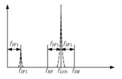
The preceding figure shows the transfer of phase noise from  $f_{LO1}$  to  $f_{IF1}$ .
