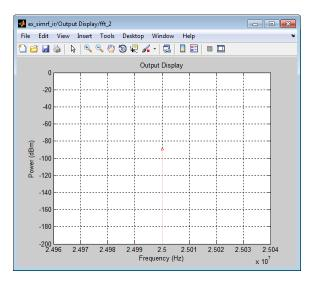
As expected, the system removes the image and amplifies the RF by 6 dB.
