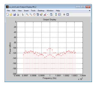
The quantization error exceeds the receiver noise.
