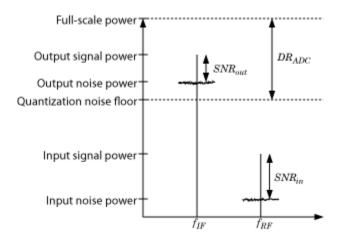
The preceding figure illustrates an RF signal that falls within the dynamic range (DR) of an ADC. The input signal and noise at the carrier  $f_{RF}$  has high signal-to-noise ratio (SNR). The received signal at  $f_{IF}$  has reduced SNR due to system noise figure. However, if the quantization error is near or above the receiver noise, system performance degrades.
