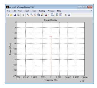
The Sinusoid source generates a two-tone signal centered at  $f_{IM}$ .
