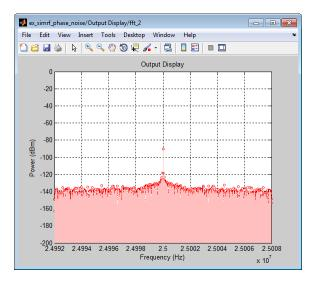
The LO phase noise has been transferred to the receiver output. The peak signal power is the same as in the previous section, "Create a Model with RF Interference" on page 2-2.
