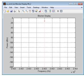
The power level of the blocker is about 90 dB higher than the signal power of the RF..
