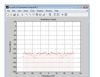
• The Quadrature Output plot shows the power spectrum of the quadrature signal at baseband.
