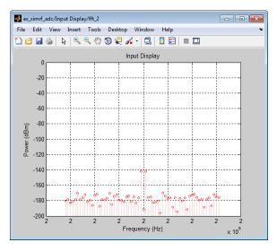
The measured power of each tone of -142 dBm is consistent with the expected power level of a .1- $\mu$ V signal. The power level of the noise is consistent with a -174 dBm/Hz noise floor.
